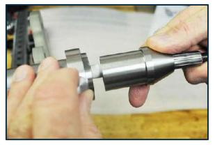
3.) Push the guide fully into the extension tube and secure it with the locking screw.
