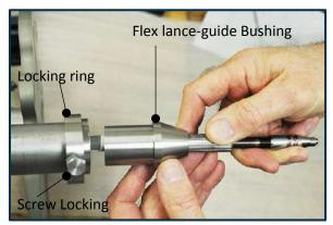
2.) Check that the locking screw is sufficiently unscrewed to permit the lance guide to slide completely into the extension tube.
